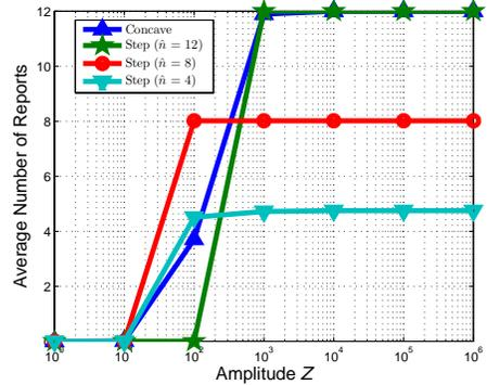
Fig. 6. The average number of reports received by the SP versus amplitude  $Z$  in different utility functions. We assume that  $I_l = 12$ ,  $c_i = 8$ ,  $\sigma_i \in \mathcal{N}(5, 1)$ , and  $p_i^{\text{nowifi}}(T) \in U[0.1, 0.9]$ .
