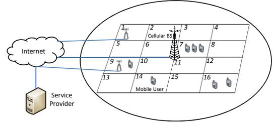
Fig. 1. An example of the network setting, where the users are moving within a set of  $\mathcal{L} = \{1, \dots, 16\}$  locations. The users are always under the coverage of a cellular base station, but Wi-Fi is only available at locations 1 and 9.
