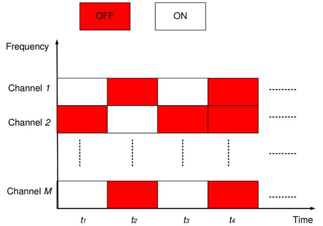
Fig. 2. Channel model of the cognitive radio network.
