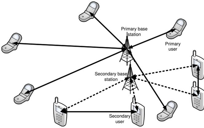
Fig. 1. A cognitive radio network scenario. In the secondary network, the dotted arrows denote the control channels between the secondary base station and the secondary users, and the solid arrows denote the data channels used (either between the primary base station and primary users, or between a secondary transmitter and a secondary receiver).
