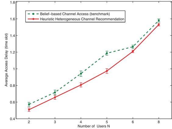
Fig. 11. Average access delay of channel recommendation and belief-based channel access (benchmark) schemes with heterogeneous channel data rates
