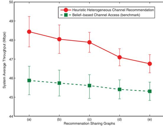
Fig. 13. System average throughput of channel recommendation and belief-based channel access (benchmark) schemes with different recommendation sharing graphs
