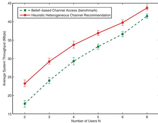
Fig. 10. System average throughput of channel recommendation and belief-based channel access (benchmark) schemes with heterogeneous channel data rates
