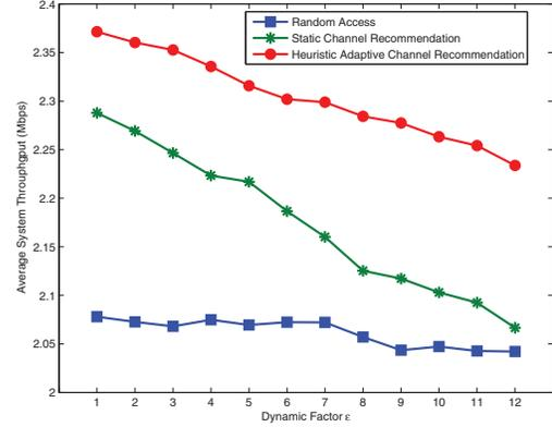
Fig. 4. Comparison of three channel access schemes
