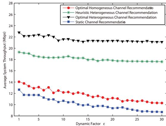
Fig. 8. Comparison of heuristic heterogeneous channel recommendation, optimal homogeneous channel recommendation and optimal homogeneous channel recommendation
