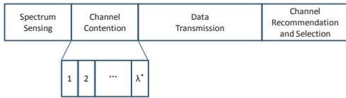
Fig. 2. Structure of each spectrum access time slot
