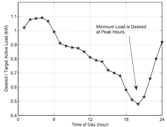
Fig. 5. An example target active power consumption level to be announced by utility / aggregator in a command-based CFVR system. The commands aim to push the load from peak hours to off-peak hours.
