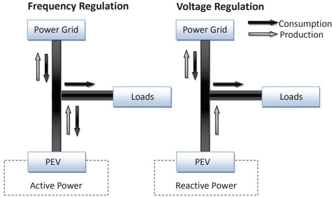
Fig. 1. System model for PEV-based combined frequency and voltage regulation.
