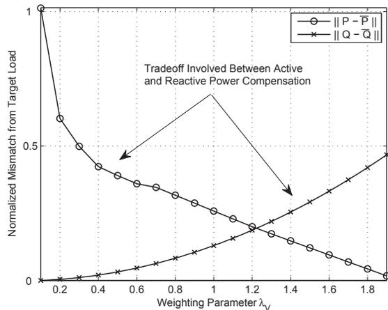
Fig. 6. Trends between  $\lambda_V$  versus the active power mismatch  $\|P - \bar{P}\|$  and the reactive power mismatch  $\|Q - \bar{Q}\|$ .
