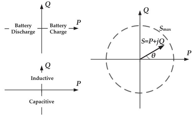
Fig. 2. Four-quadrant power response of a PEV [1].
