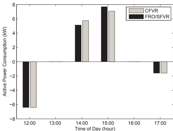
Fig. 7. Comparisons of active power scheduling profile among FRO, SFVR and CFVR using level 2 charging.
