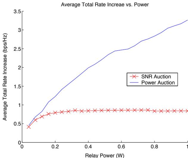
Fig. 7. Total network rate increase vs. relay power.
