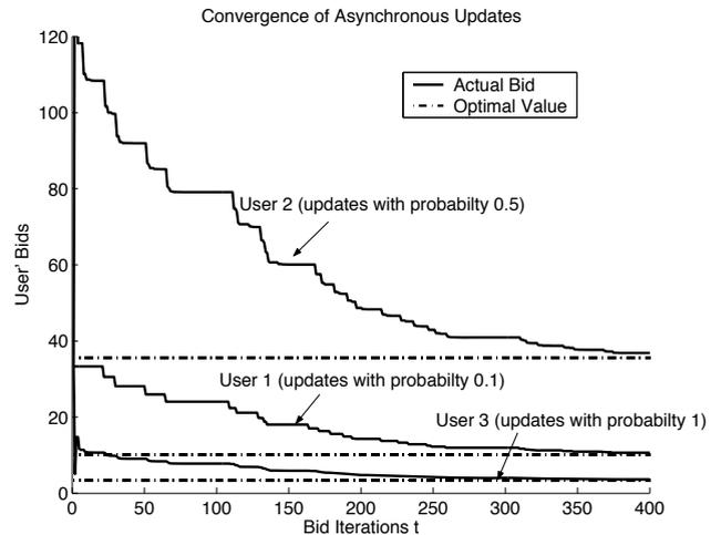
Fig. 9. Convergence of bids under asynchronous updates.
