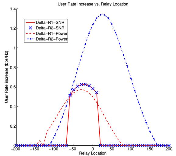
Fig. 5. Individual rate increase vs. relay location (y-axis) for an SNR auction and a power auction (users have equal weights in the SNR auction).
