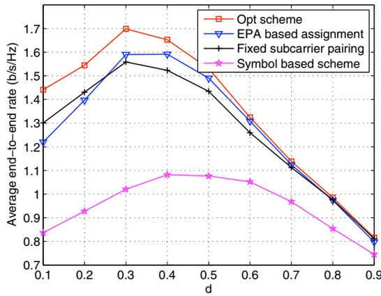
Fig. 4. Comparison of average end-to-end transmission rate versus relay location. Power per node = 20dBW.
