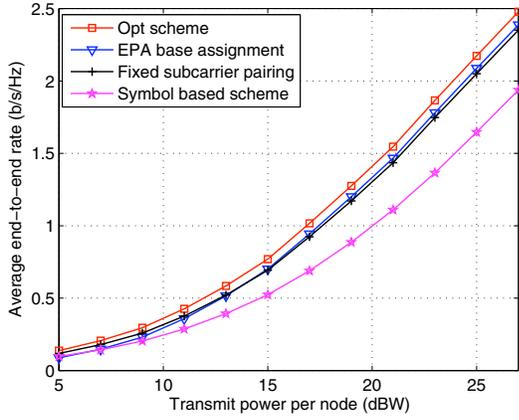
Fig. 3. Comparison of average end-to-end transmission rate versus transmit power per node.
