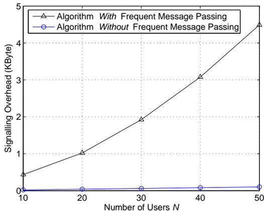
Fig. 4. Comparison between Algorithm 1 in [9] (i.e., the algorithm *with* explicit message passing) and our proposed Algorithm 1 (i.e., the algorithm *without* explicit message passing) in term of the signalling overhead when the number of users varies from 10 to 50.
