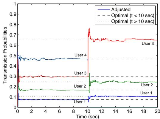
Fig. 2. Simulation results for Algorithm 1 when  $\alpha = 0.6$ . The number of users and the features of the communication channel change after  $t = 10s$ . The optimal transmission probabilities before  $t = 10s$  (i.e., dashed lines) and after  $t = 10s$  (i.e., dotted lines) are obtained using [9, Algorithm 1].
