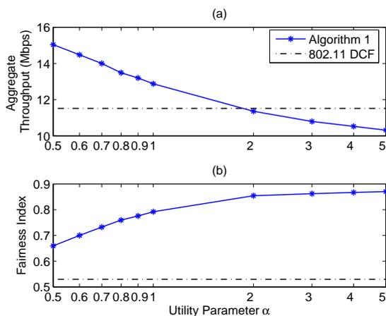
Fig. 5. Comparison between Algorithm 1 and 802.11 DCF when  $N = 10$ .
