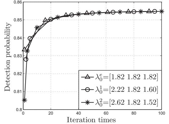
Fig. 2: Detection probabilities converge with different IDTs.
