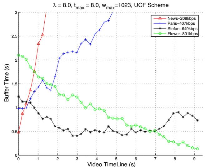
**Fig. 6.** Four users simulation for under-served Situation by UCF
