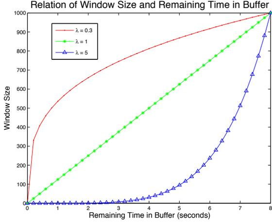
**Fig. 2.** Back off window size as function of buffer time
