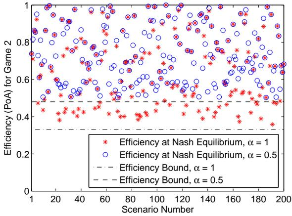
Fig. 4. Efficiency (PoA) at a Nash equilibrium of 200 randomly generated resource allocation game scenarios when the network topology is as in Fig. 2,  $N = 2$ . Here we set either  $\alpha = 1$  or  $\alpha = \frac{1}{2}$ . For each scenario, utility functions  $U_1$  and  $U_2$  as well as the pricing parameter  $a$  are selected randomly.
