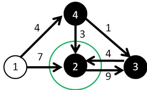
Fig. 1. A GSCG. The users are represented by vertices in a weighted graph. Users suffer interference from other users of the same channel which are connected to them. For example, user 2 suffers an interference level of 3 from user 4 (which is also using the *black* channel), but user 2 suffers no interference from user 1 (which is using *white* channel instead).
