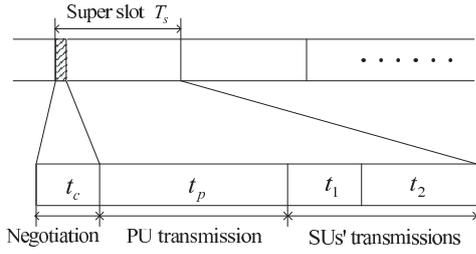
Fig. 2: Slotted structure
