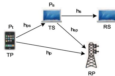
Fig. 1. The Cooperation between One PU ( $TP$ - $RP$ ) and One SU ( $TS$ - $RS$ )
