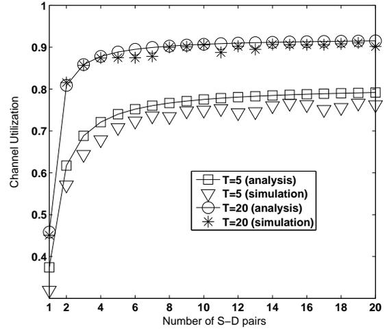
Fig. 5. Channel utilization with different number of S-D pairs.
