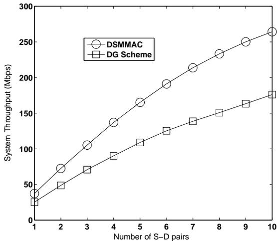
Fig. 10. System throughput with different number of S-D pairs.
