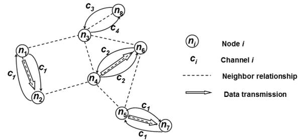
Fig. 1. A generic multi-channel wireless network with 8 nodes and 4 channels.
