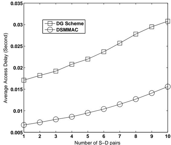
Fig. 11. Medium access delay with different number of S-D pairs.
