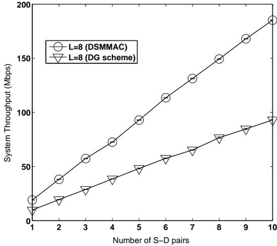
Fig. 6. System throughput with different number of S-D pairs.
