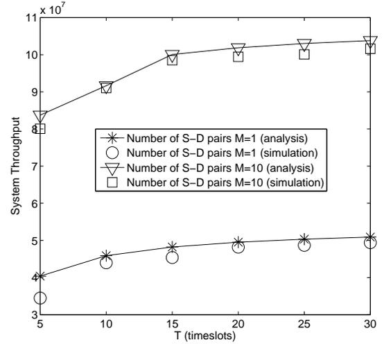
Fig. 4. System throughput versus duration of each data transmission.
