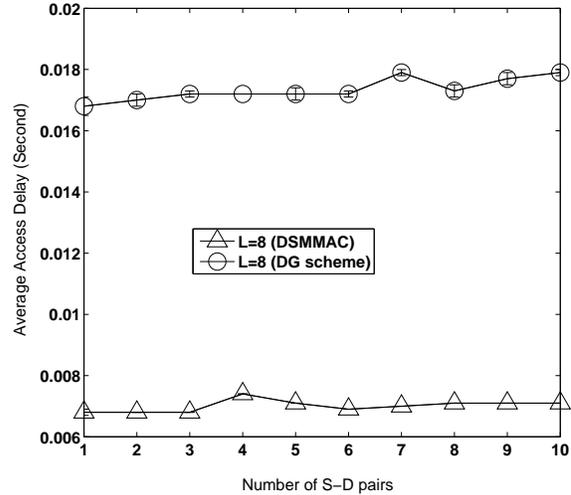
Fig. 7. Medium access delay with different number of S-D pairs.
