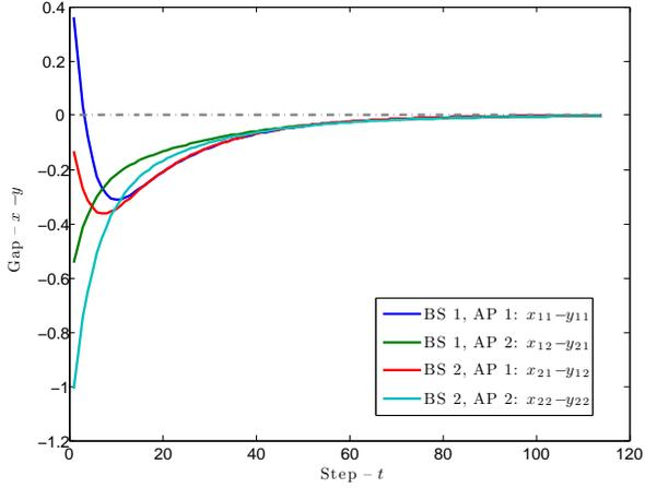
Fig. 4. Evolution of the gap between the requested data traffic by BSs ( $x$ ) and the admitted by APs ( $y$ ).
