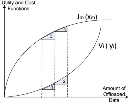
Fig. 2. Concave BS utility function,  $J_m(\cdot)$ , and convex AP function,  $V_i(\cdot)$ . The numbered triangles have the same length - corresponding to equal offloaded data increase - but different height ( $h$ ):  $h_2 > h_1$  and  $h_4 < h_3$ .
