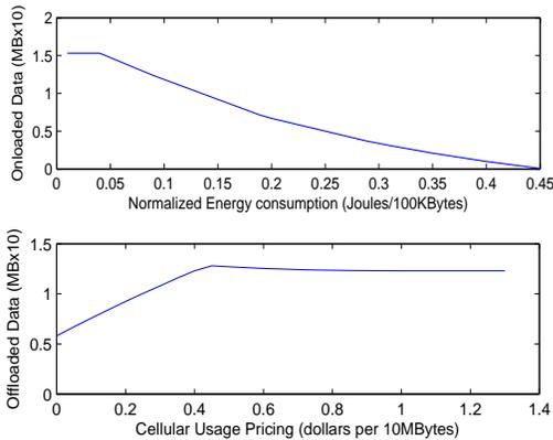
Fig. 5. Upper subfigure (Onloading): 4G capacity (10 Mbps) is 5 times larger than the WiFi capacity (2 Mbps), mobile data price is  $p = 0.01$  \$/Mbit, and the 4G link energy consumption 3-times larger than the WiFi link energy consumption ( $e_{0i} = 2.85$  J/MB). Lower subfigure (Offloading): 4G capacity (4 Mbps) is twice the WiFi capacity, and data usage price increases.
