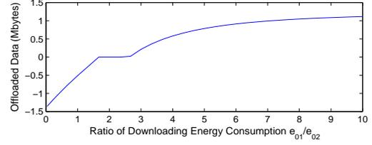
Fig. 6. Offloading - onloading decisions based on the energy consumption ratio  $e_{01}/e_{02}$  for the 4G user (user 1) and the WiFi user (user 2). Cellular data usage is free of charge, and 4G capacity is twice the WiFi capacity (2Mbps).
