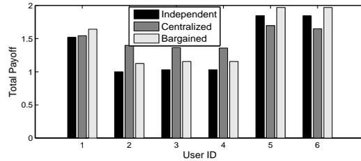
Fig. 3. Comparison of centralized, independent, and bargained solution. System basic parameters are:  $\{C_{0i}\}_i = \{12.7, 0.0, 1.0, 1.0, 4.12, 2.1\}$  Mbps,  $\{e_{0i}\}_i = \{0.58, 0.0, 12.5, 12.5, 0.36, 0.36\}$  Joule/Mbit, and  $\{p_i\}_i = \{0.02, 0, 0.008, 0.001, 0.0, 0.0\}$  \$/Mbit. The aggregate total payoff improvement of the bargained solution (compared to the independent solution) is approximately 10%.
