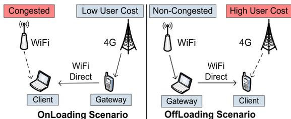
Fig. 2. The service can be used to *offload* cellular traffic to WiFi access points (AP), or *onload* WiFi traffic to cellular networks (downloading scenario). The offloading decisions depend mainly on the data usage (and energy) cost incurred by the users (user-initiated offloading), while the onloading decisions depend on the congestion of WiFi APs.
