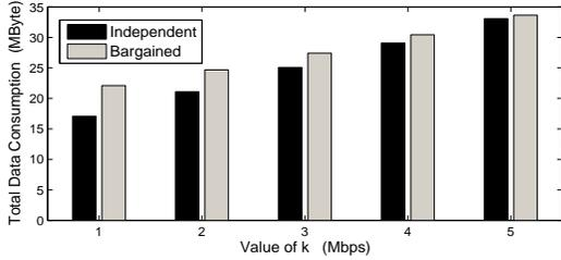
Fig. 4. Service performance for users with diverse Internet access capacities.  $C_{01} = C_{02} = 12.7$  Mbps,  $C_{03} = C_{04} = C_{05} = C_{06} = k$  Mbps. Internet access prices are identical and equal to  $p = 0.01$ . Similarly, energy consumption for downloading is  $e_{0i} = 0.158$  for each user  $i$ . Results are averaged over 30 runs with uniformly distributed user locations in  $[0, 100m] \times [0, 100m]$ .
