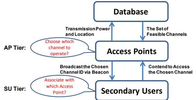
Fig. 1. System architecture of AP-based white-space networks.
