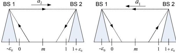
Fig. 2. Illustration of the access pricing. Left: To complete an inter-network traffic initiated from network 1, network 2 charges network 1  $a_2$  per unit of bandwidth. Right: the access price  $a_1$  is defined similarly.
