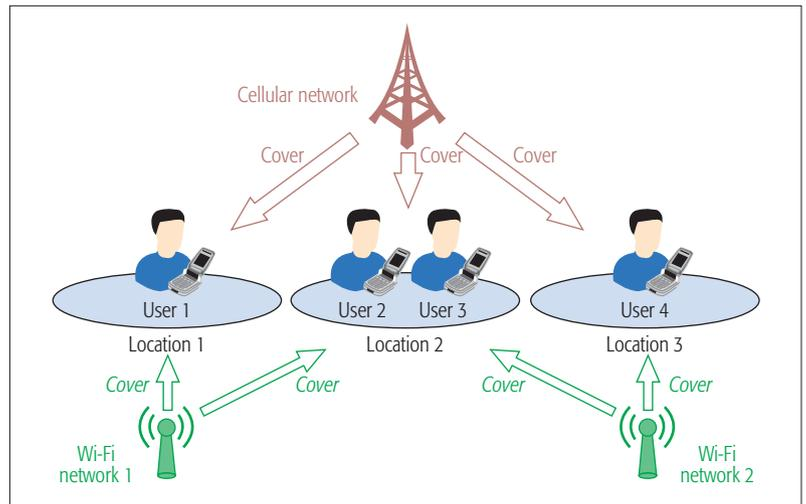
FIGURE 2. An example of the system model, where users 1, 2, 3, and 4 are moving among locations 1, 2, and 3. The cellular network covers all locations. Wi-Fi network 1 covers locations 1 and 2, and Wi-Fi network 2 covers locations 2 and 3.
