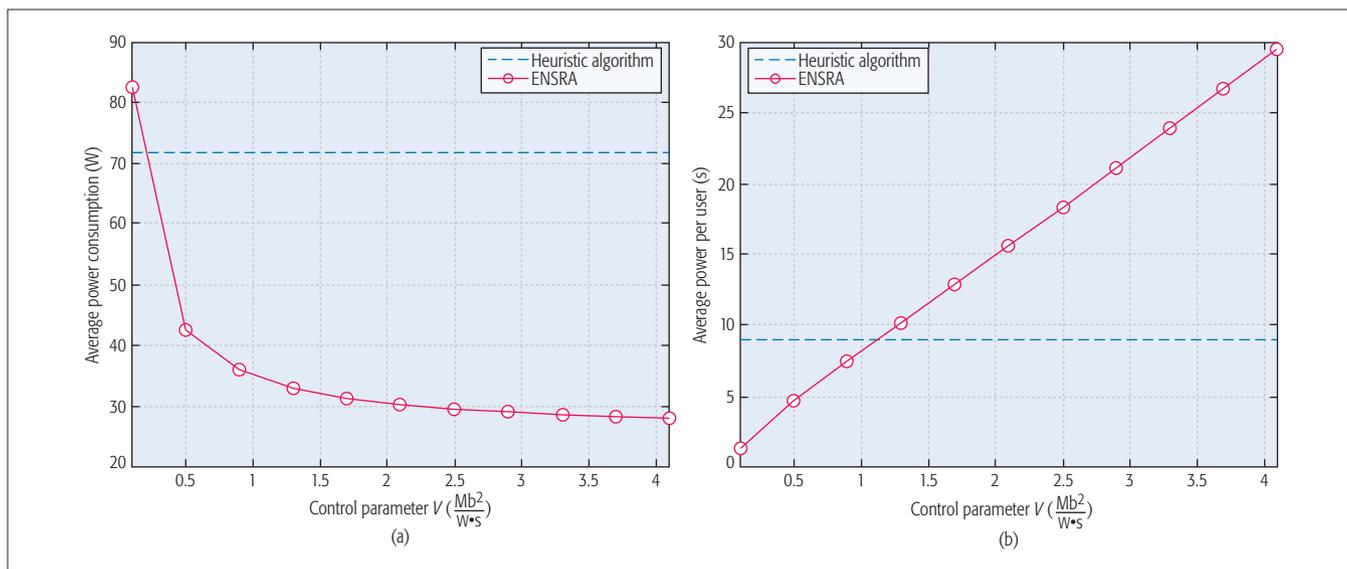
FIGURE 3. Comparison of ENSRA and heuristic algorithm: a) power consumption vs. parameter  $V$ ; b) traffic delay vs. parameter  $V$ .
