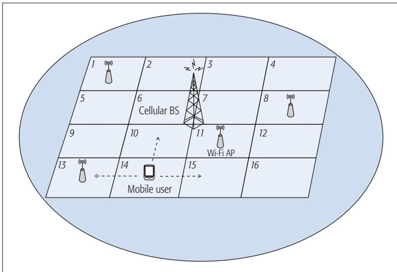
FIGURE 5. An example of the network setting, where a user is moving within 16 locations. The user is always under the coverage of a cellular base station, but Wi-Fi is only available at locations 1, 8, 11, and 13.
