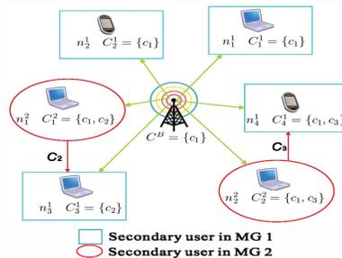
Fig. 1. The illustration of cooperative transmission for multicast service in heterogeneous cognitive radio network.
