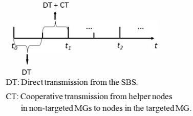
Fig. 2. The illustration of enhancement layer transmission in time domain.
