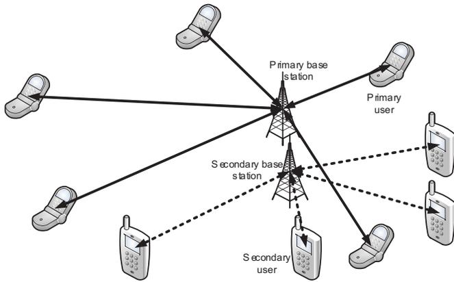
Fig. 1. A cognitive radio network scenario. In the secondary network, the dotted arrows denote the channels between the secondary base station and the secondary users.
