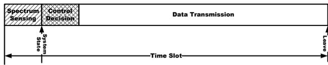
Fig. 2. The components of a time slot.
